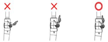
Please make sure that the rear suspension joint must be completely locked to the end correctly. Any extra push and pull will not move it unless the safety lock is properly released according to the correct unlocking steps. Please be sure to confirm it carefully, otherwise there will be an accidental risk.
